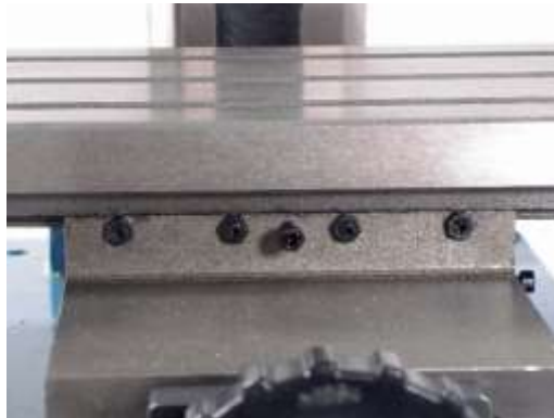
X-axis gib adjusting screws
